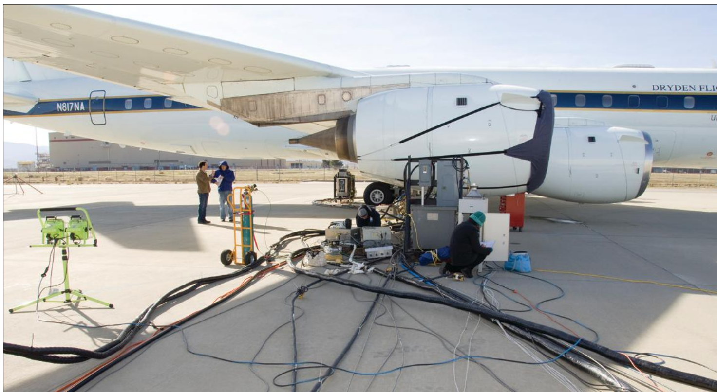
A maze of wires and tubing that connects data-collection instrumentation to the control centers is laid out on the pavement beside the DC-8 flying laboratory during synthetic fuels emission and performance testing.
