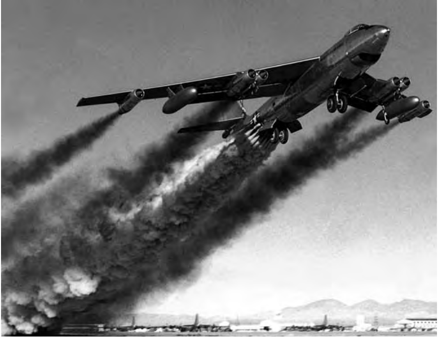
Air pollution is evident as this Boeing B-47B takes off in 1954 with the help of its General Electric J47 jet engines and Rocket Assisted Take Off solid rocket motors. U.S. Air Force.
