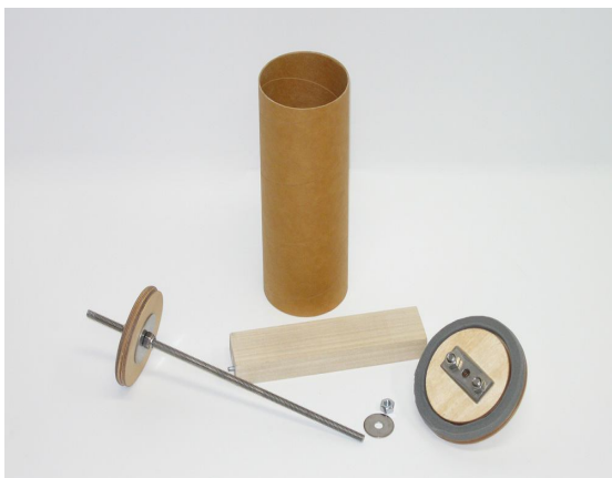
Basic altimeter bay components - aft bulkhead, through-bolt, coupler and forward bulkhead
