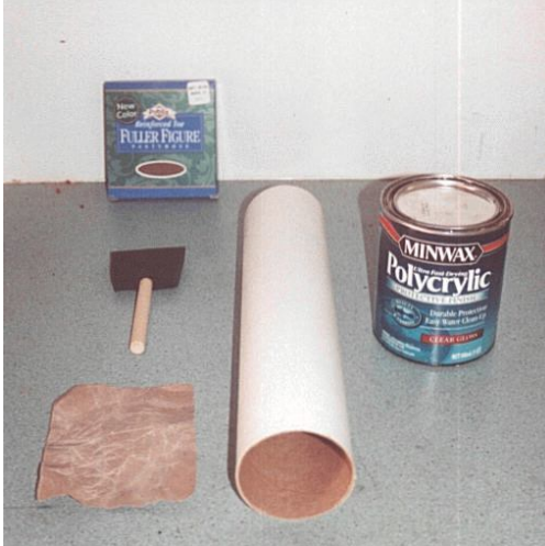
Quasi-Glass components: Tube, Plus-size pantyhose, 2" foam brush, sandpaper, Miniwax Polycrylic finish
