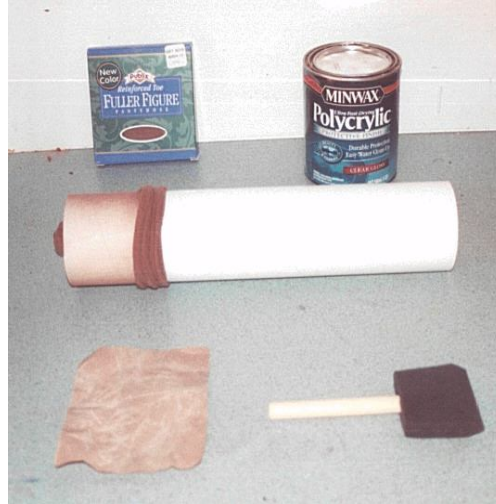
Quasi-Glass components: Tube, Plus-size pantyhose, 2" foam brush, sandpaper, Miniwax Polycrylic finish
