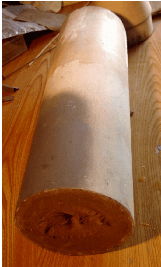
Nylon hose applied to 5.5" LOC tube
