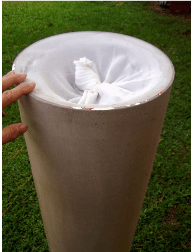
An 11.5" PML tube with 8" Drain-Sleeve after application of Polycrylic clearcoat
