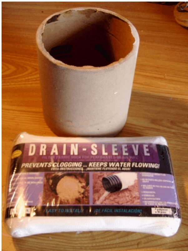
A scrap piece of 5" cardboard Uline tube after covering with 4" Drain-Sleeve
