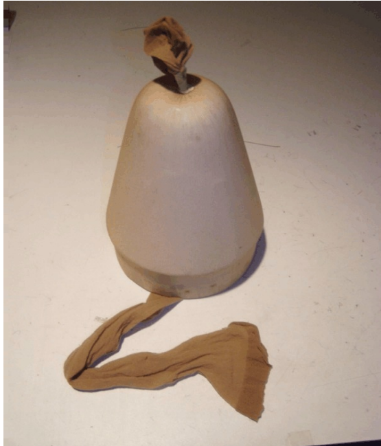
Covering a strap-on booster cone for Long March scale model with nylon hose, demonstrating application of Quasiglass method to nose cones
