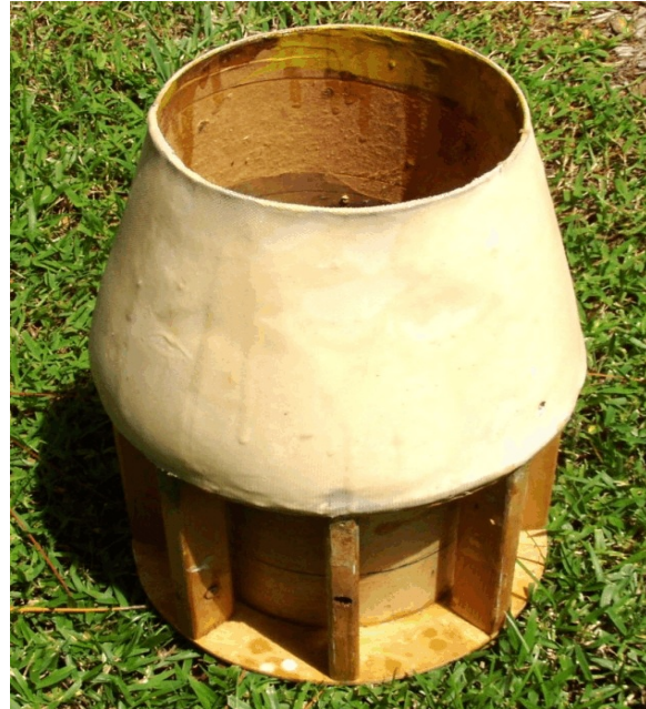
A scratchbuilt 11.5"-to-7.5" transition section, with posterboard surface covered with 8" Drain-Sleeve, Polycrylic and a coat of laminating epoxy
